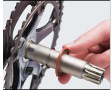
Figure 25. Sliding the wave washer and bearing cover onto the axle
